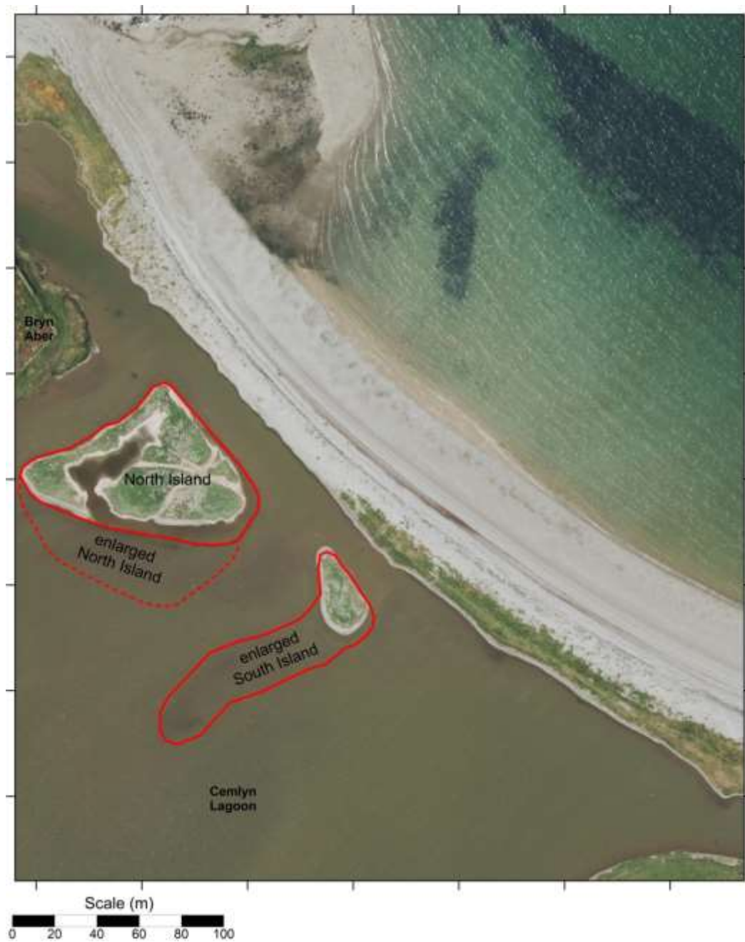
Figure 22. One possible option to increase the surface area of the tern islands using imported sediment . Base aerial photography flown spring 2014 (from Pye & Blott, 2018a)
