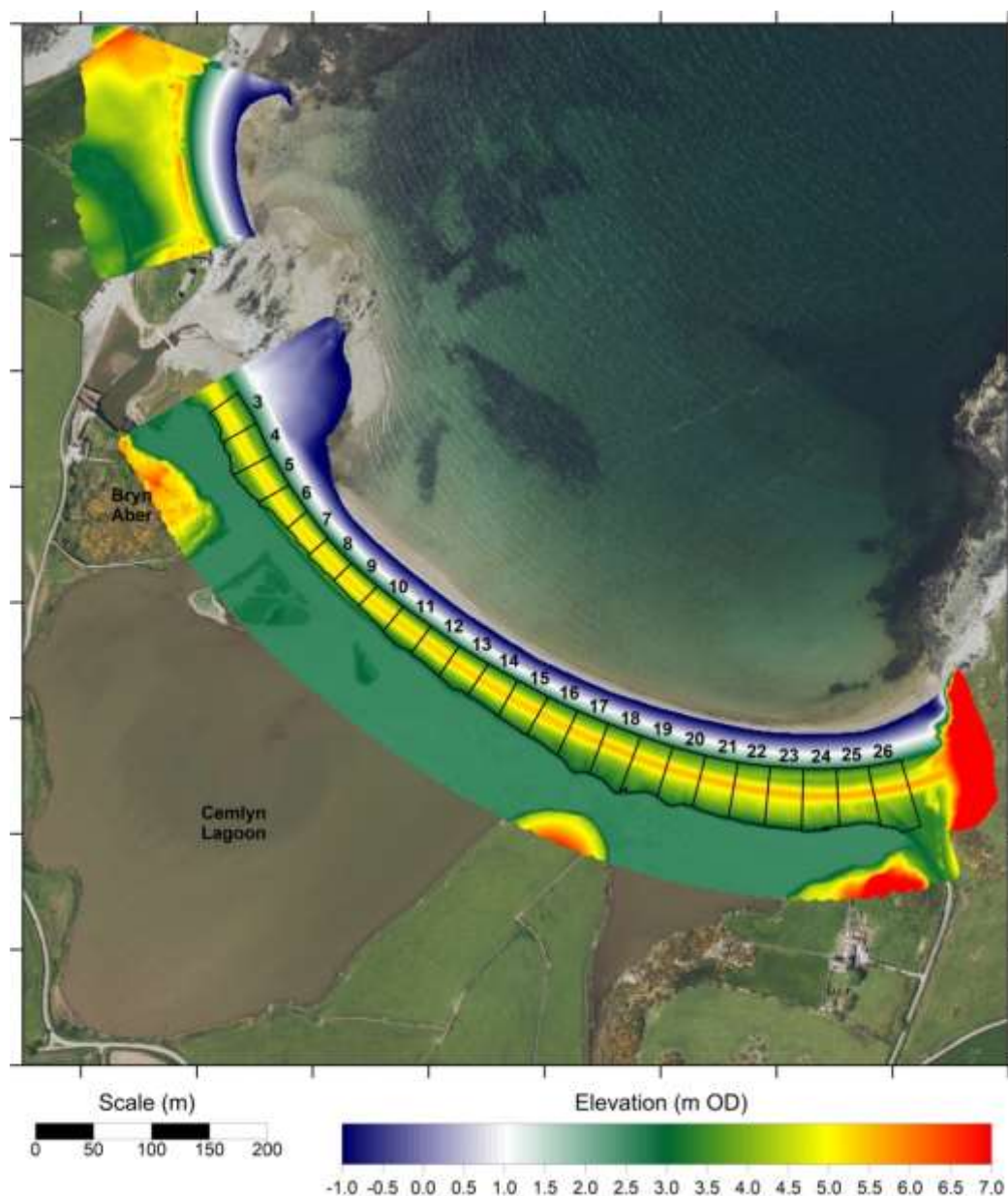
Figure 21. Modified terrain model of the shingle ridge after hypothetically increasing the height and volume to match the ridge profile in Cell 12, and with an assumed ridge crest elevation of 5.2 m ODN at NW end and 5.7 m ODN at SE end (from Pye & Blott, 2018a)
