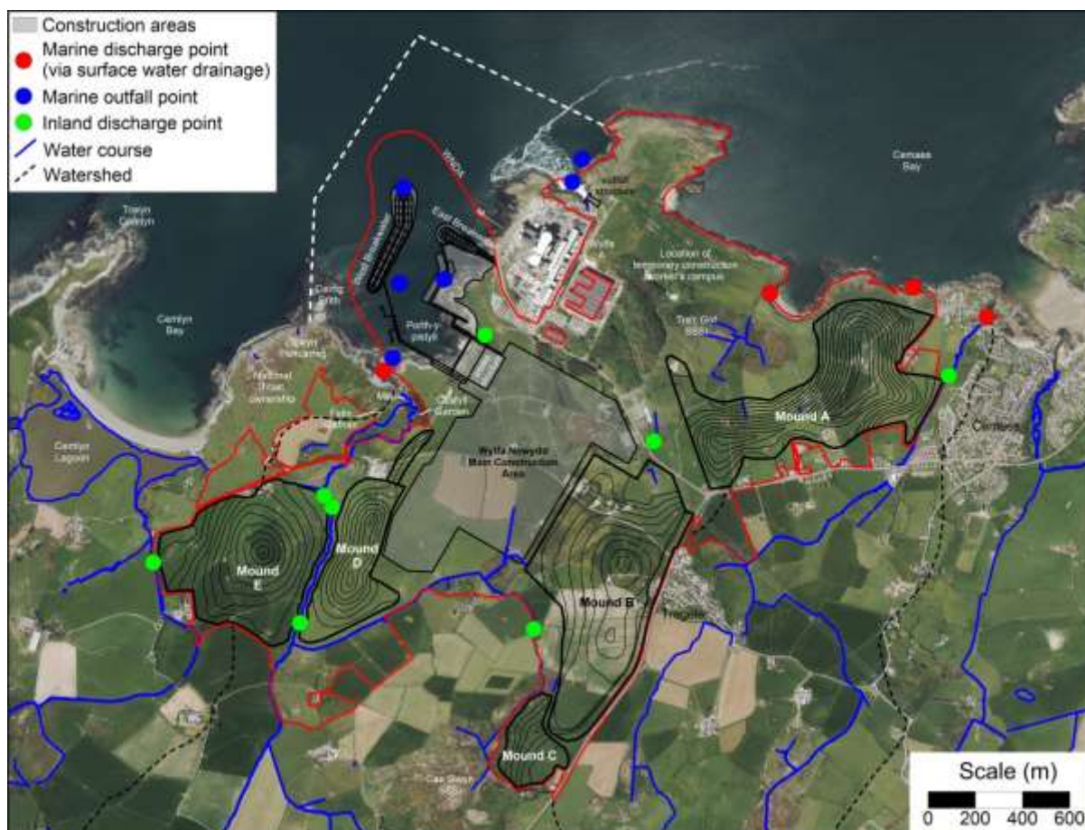
Figure 3. Proposed location of earth mounds, drainage routes and discharge points within the WNDA, also showing extent of proposed harbour works (indicative boundary of statutory harbour limits shown by the white dotted line); Project information taken from DCO documents and superimposed on base 2014 aerial photography
